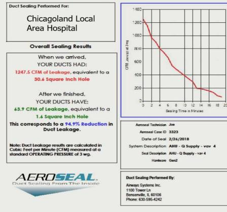
When we arrived YOUR DUCTS HAD: 1,247.5 CFM of Leakage equivalent
